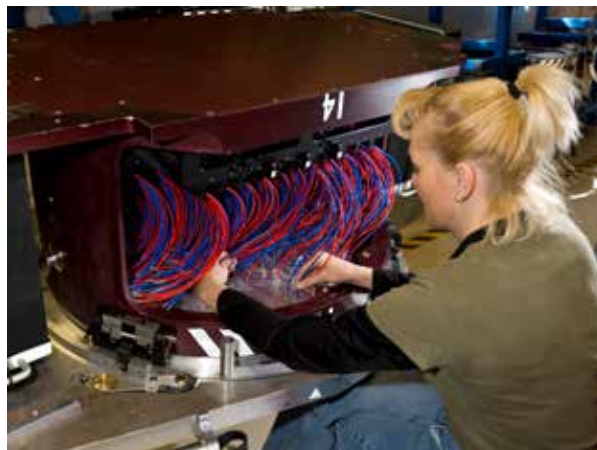
SDSS technician Diana Holder at the Apache Point Observatory hand connecting optical fibers into metal plug plates to capture light during observations. (PHOTO COURTESY OF THE SDSS COLLABORATION. WWW.SDSS.ORG )
